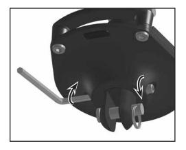
Use Blue Loctite® adhesive or alternate threadlocking solution on threads. Tighten the screws
